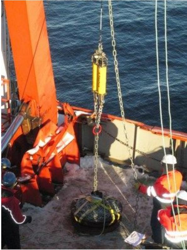
Photo 1: The anchor and the release assembly about to be lowered in the water.
