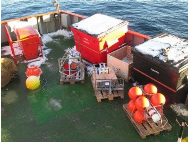
*Photo 3: Some of the instruments for the mooring; from bottom to top in the picture, you can see the location transponder (orange spheres), the ISUS instrument for measuring nitrates (black cylinder), and the ADCP (the 4 orange disks on the white cylinder).*
