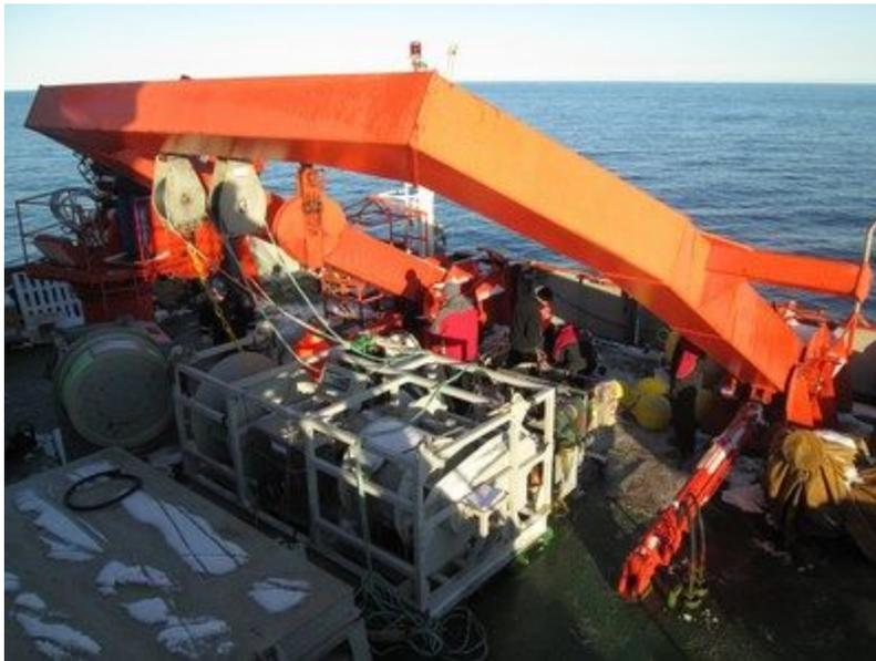
Photo 2: The mooring apparatus, about to be raised up to deploy the mooring instruments.
